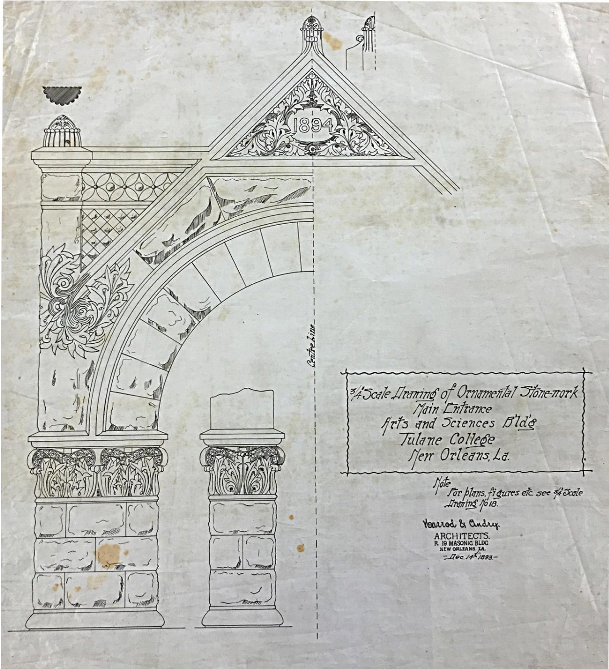
Tulane University, Arts and Sciences Building (now Gibson Hall), details for stonework. New Orleans, LA. 1893. Harrod and Andry, architects. Ink on linen.
